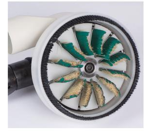
Sand-Perfect 60 is an industrial brush sanding machine developed by Flex Trim and is a powerful alternative to existing hand sanders.
