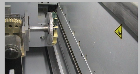
Wood sanding with disc sanders inserted in an edge sanding machine.
