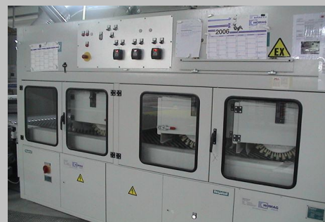
Surface sanding with a Venjakob brush sander.
