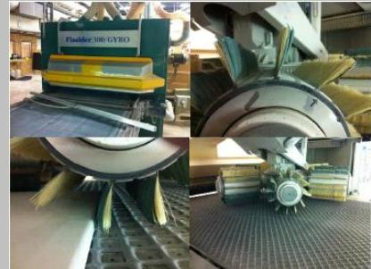
Photos from Modexa with the new inclined grooves mounted in a Fladder Gyro
