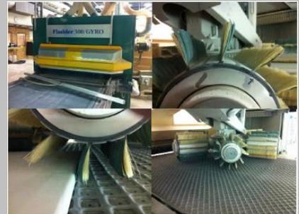
Photos from Modexa with the new inclined grooves mounted in a Fladder Gyro
