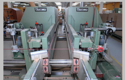
This double-end tenoner has got a Flex Trim sanding head attached.
