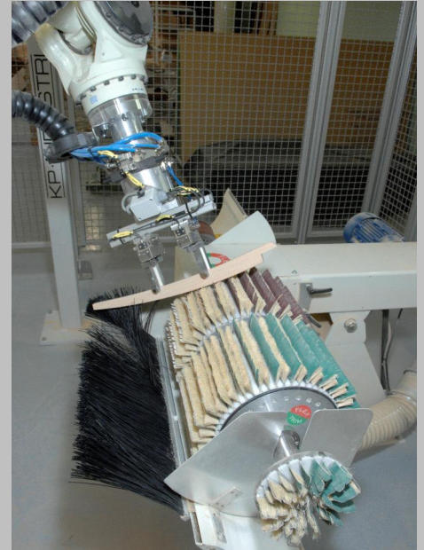
The solution from Flex Trim is here installed in a robot cell.
