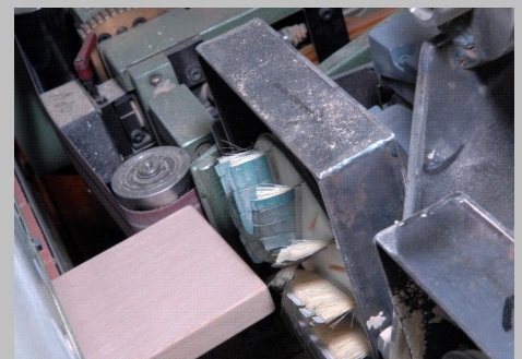
The material to be profile sanded are going past the rotating sanding head, which has an optimized rotation speed for the band speed through the double-end tenoner and the profile.
