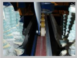
When the items are running through the adjustable machine, they are sanded on both sides and surface at the same time.
